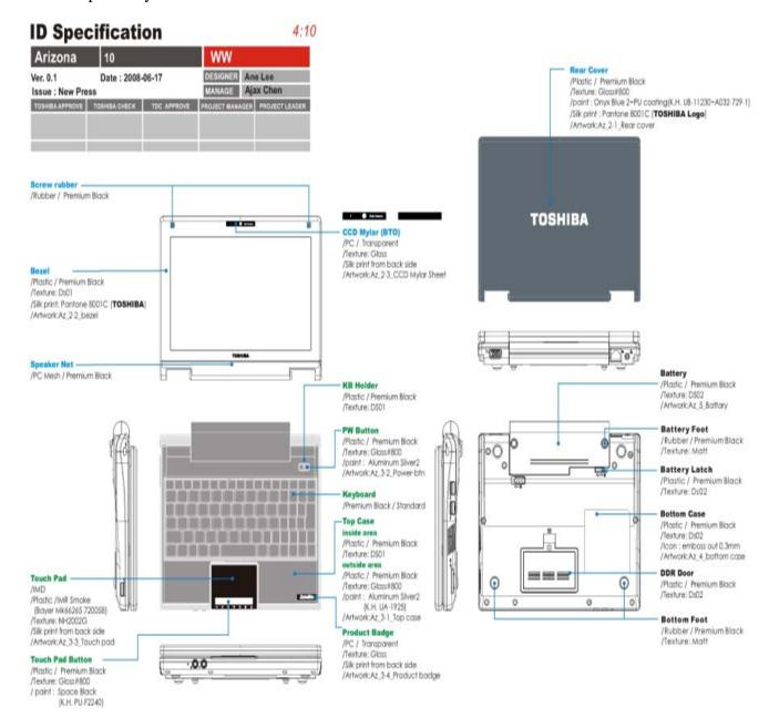
Figure 1-1 ID Parts Description Placement
